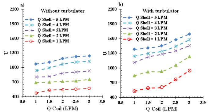
Fig. 3: Overall heat transfer coefficient for first mode (a) without turbulator b) with turbulator
