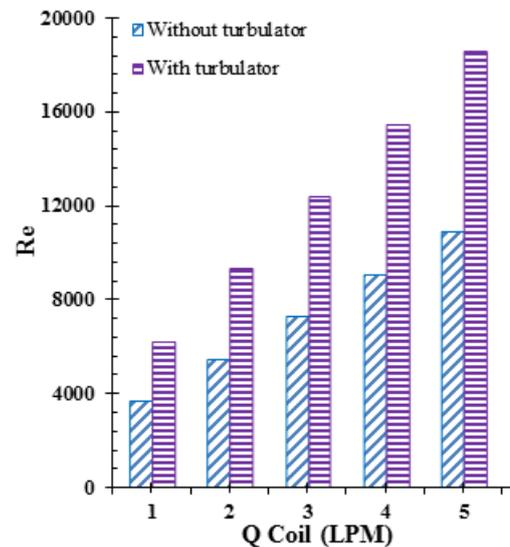
Fig. 4: Reynolds number of each flow rate for with and without turbulator
