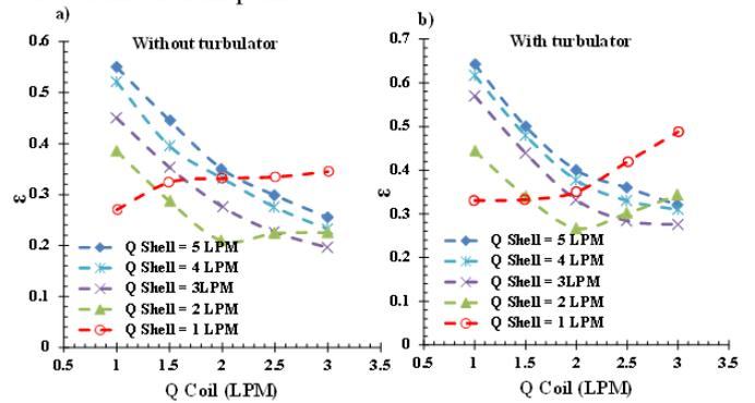
Fig. 7: Effectiveness for first mode a) without turbulator b) with turbulator
