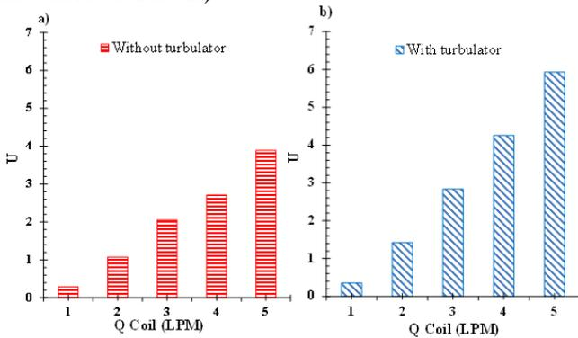
Fig. 5: Overall heat transfer coefficient a) without turbulator b) with turbulator
