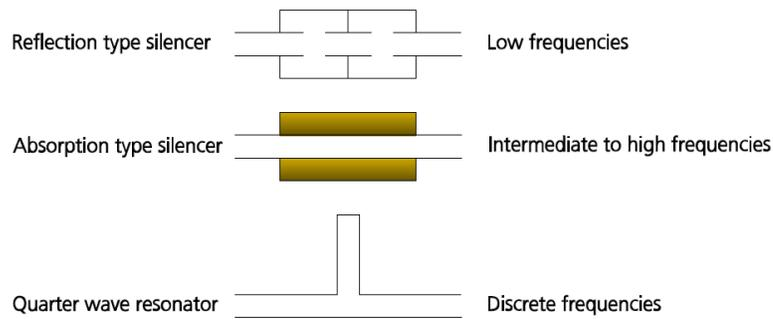
Conventional engine exhaust silencers are of the reflection type, absorption type or a combination of these two. The reflection type silencer is used for attenuating low frequencies. The absorption type attenuates the intermediate to the higher frequencies. The complete frequency range can be attenuated by a combination of the two.
