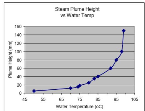
understanding of the different vapour collapsing regimes and to better understand the relationship between the steam plume and the degree of tank mixing.
