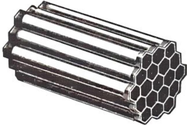
1. Due to ultrasonic vibration the heat exchanger is self-cleaning due to imposed cavitation action due to high frequency vibration and water near the boundary layer. It will automatically remove the excessive salt deposition from the vaporizing sea water (32000 ppm)
