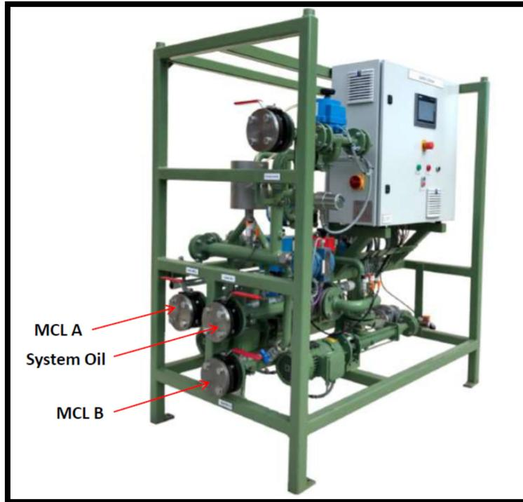
used main engine system oil with a high BN Cylinder oil to produce required cylinder oil on board. This provides a flexible composition of cylinder oil meeting varying fuel sulphur levels and engine requirements at all times, which allows for not only significantly reduced cost, but also optimised cylinder-oil feed rate, supply security, and reduced environmental impact.
