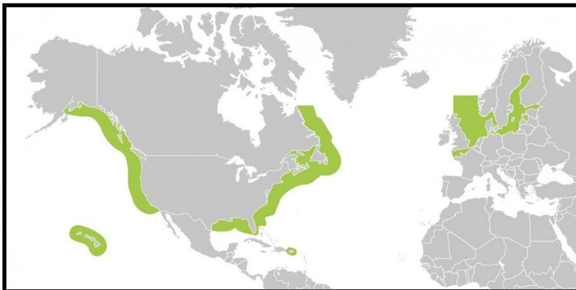
Outside of ECAs, under a new global cap, ships will have to use fuel oil on board with a sulphur content of no more than 0.50%, against the current limit of 3.50% (Fig.2). Ships may also meet the SO<sub>x</sub> emission requirements by using approved equivalent methods, such as exhaust gas cleaning systems (EGCS) or “scrubbers”, which “clean” the emissions before they are released into the atmosphere.
