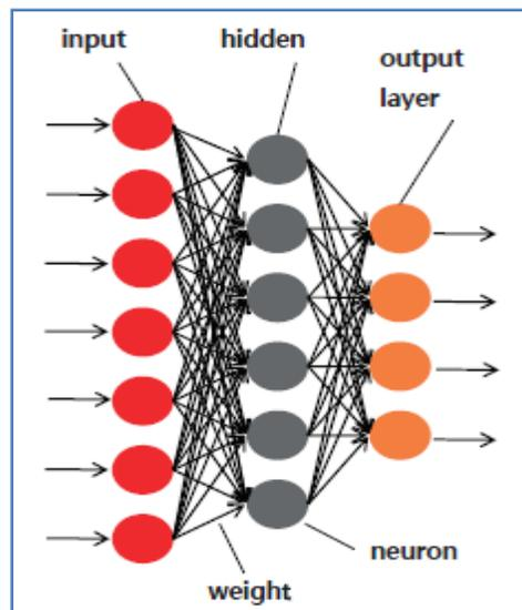
**Fig 2 Feed-Forward Neural Network with one Hidden Layer**
