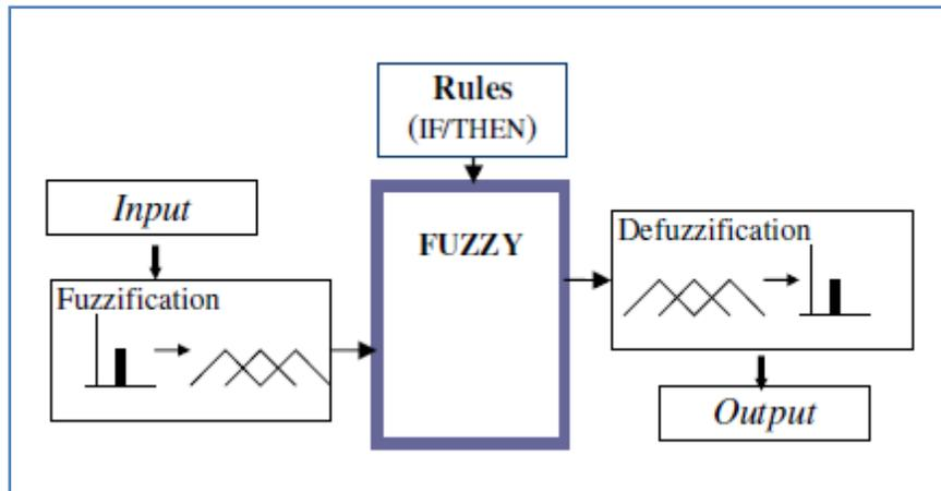
**Fig 3 Fuzzy Logic Diagnostic System**
