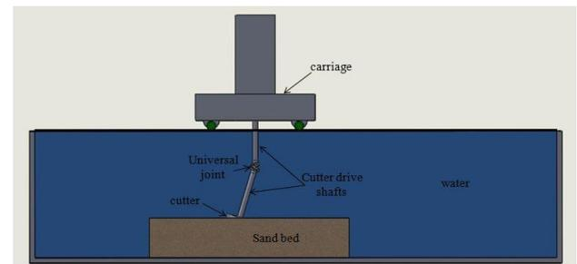
Fig 2: Equivalent model for the dredging operation
