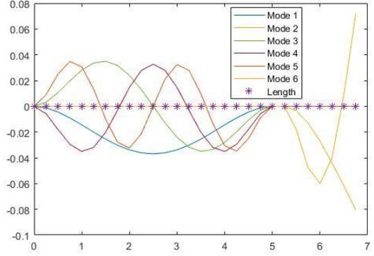
Fig 6: Modeshapes of the system due to added mass effect with high stiffness at the joint
