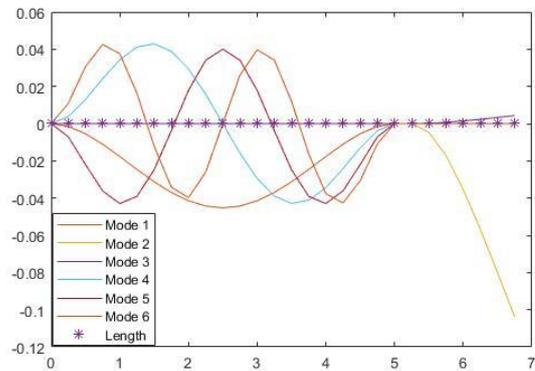
Fig 5: Modeshapes of the system with high stiffness at the joint
