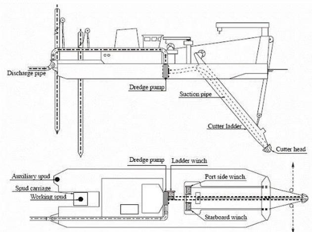
Fig 1: the top view and front view of the cutter suction dredger. [6]
