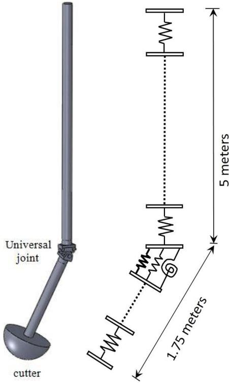
Fig 3: Diagram of cutter drive with cutter, its spring equivalent system
