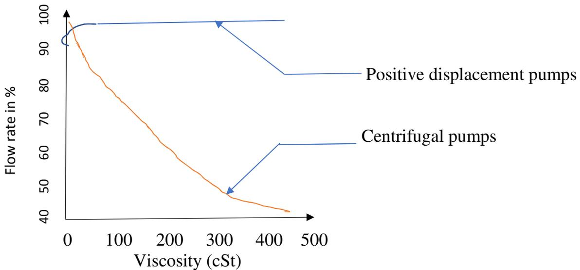
**Figure 5: - flow rate vs. viscosity**
