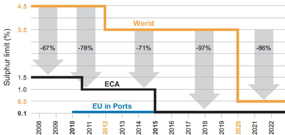
**Figure 1: - Step down reduction in Sulphur limits**
